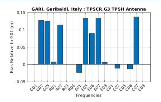
Note the interfrequency bias is different for different antennas
