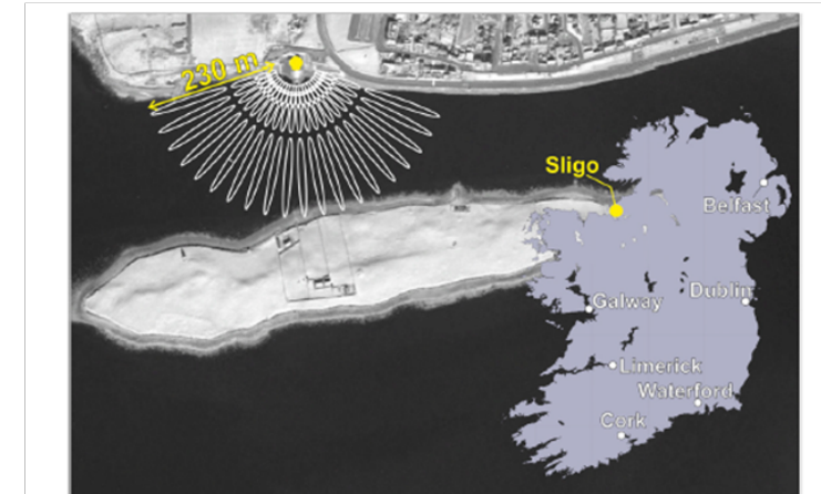
FIG. 1. Satellite view of the Sligo test site (solid yellow circle) with Fresnel zones for a reflector height of 16m and elevation angles of 5° (largest white ellipses), 10°, 15°, and 20° (smallest ellipses) within the azimuth range 110°-251°.
